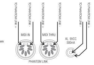
The two plugs: DIN 7 poles and coaxial 2,5mm are connected concerning the power supply (pin1 and pin7).
